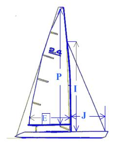
Areas of Sail Mainsail  $0.5 \times P \times E =$  $m^2$ Foretriangle Total  $0.5 \times I \times J =$  $m^2$ Foretriangle Total x 0.85 m<sup>2</sup> Sail Area For Rating = S = $m^2$  $\sqrt{\mathbf{S}}$ Builder Designer ..... When Built..... Measured by..... Date of Measurement ..... Complementary measured by..... Date of compl measurement.....
